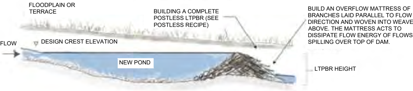
EXAMPLE LOW TECH PROCESS BASED RESTORATION PROFILE VIEW NTS
