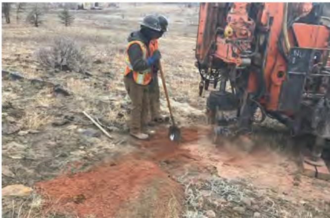
**PHOTOGRAPH 23** Clinker cuttings from MM-47, looking north.
