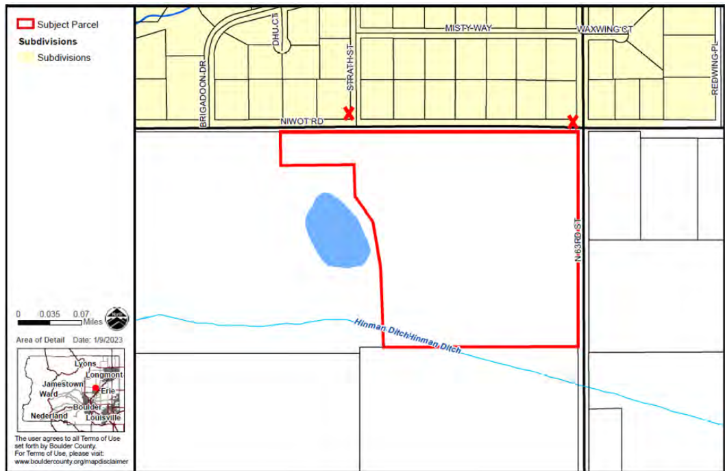
Figure 4. Subject parcel with existing fire hydrants indicated by red Xs.
