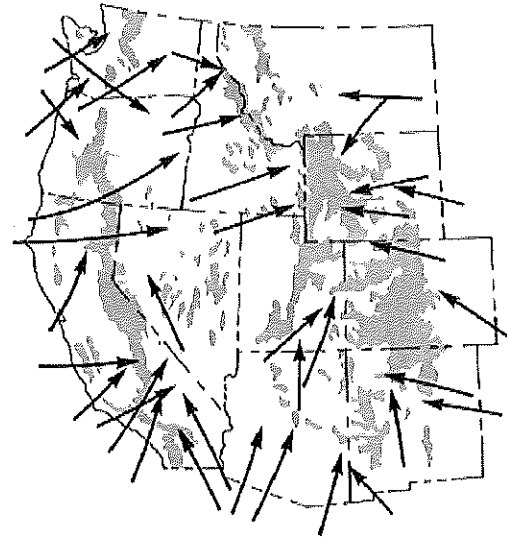
Figure 7. Principal paths of moisture inflow in the western United States for storms producing large precipitation amounts. Toned areas are major orographic barriers.
