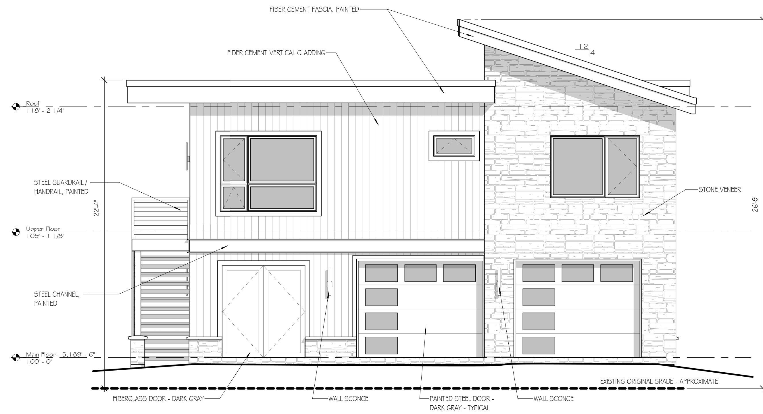
1 North Exterior Elevation 1/4" = 1'-0"
