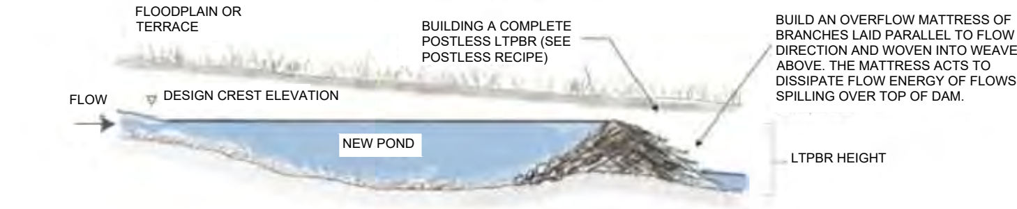
EXAMPLE LOW TECH PROCESS BASED RESTORATION PROFILE VIEW NTS
