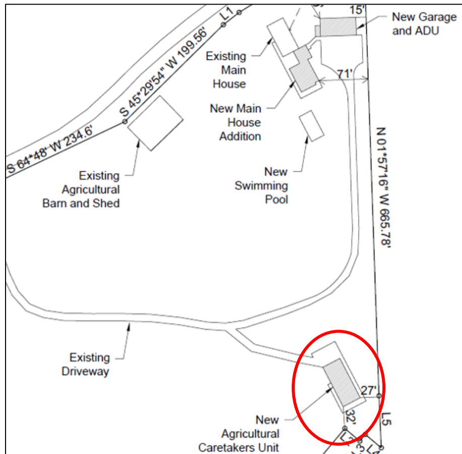
Figure 9: Detail of site plan, with proposed location of the Agricultural Worker ADU indicated in red.
