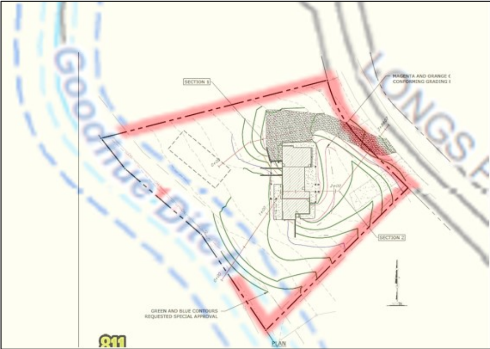
Figure 7: Proposed grading plan overlaid on zoning map with ditch setback.
